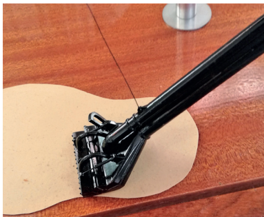
Schaalmodel sleephopperzuiger Volvox Olympia. Scale model of trailing suction hopper dredger.
