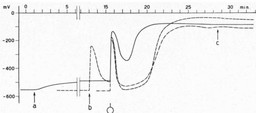
Fig. 3. Influence of oxygen. Three different vessels. At moment *a*, nitrogen plus 0.2% oxygen was passed through the suspension. At *b*, a solution of 6 mm<sup>3</sup> oxygen in water was added. At *c*, a solution of 0.25 mg catalase was added.
