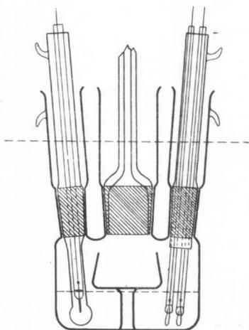
Fig. 1. Diagram of manometer vessel adapted to the measurement of pH and oxidation-reduction potential.
