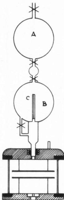
Fig. 1. Scheme of the gasdischarge chamber with glass bulbs. A is filled with pure oxygen. B is the expansion bulb. C capillary for regulation of the pressure in the discharge chamber.
