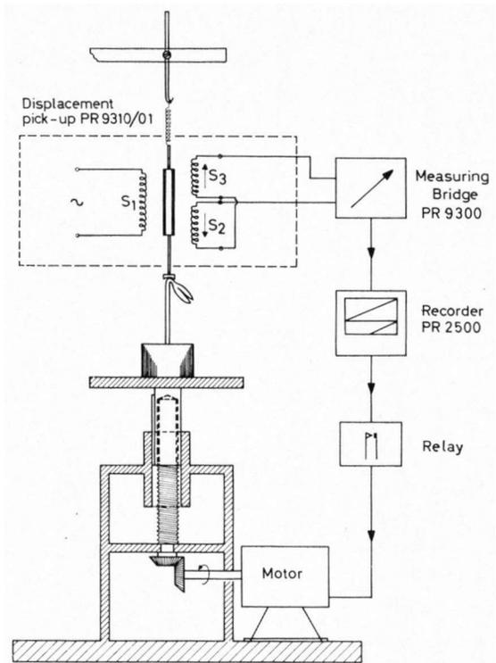
recorder pen switches on a motor. The table on which the plant is fixed moves down over 1mm, the motor is switched off when the recorder pen reaches the beginning of the scale. In this way growth can be recorded for a longer period.
