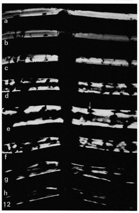
to be related to the presence of an S3 layer in the normal wood, and of the denatured remains of the cytoplasm (WARDOP & HARADA 1963). An example of the attack of cellulase on isolated fibres or tracheids is illustrated in figs. 12 a-h on Scots Pine.
