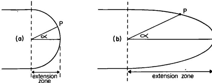
Fig. 1. The rate of expansion of any point at the apex is proportional to the cosine of the angle  $\alpha$  when the shape of the tip is hemispherical (a), or to the co-tangent of the angle  $\alpha$  when the shape of the tip is half ellipsoid (b).
