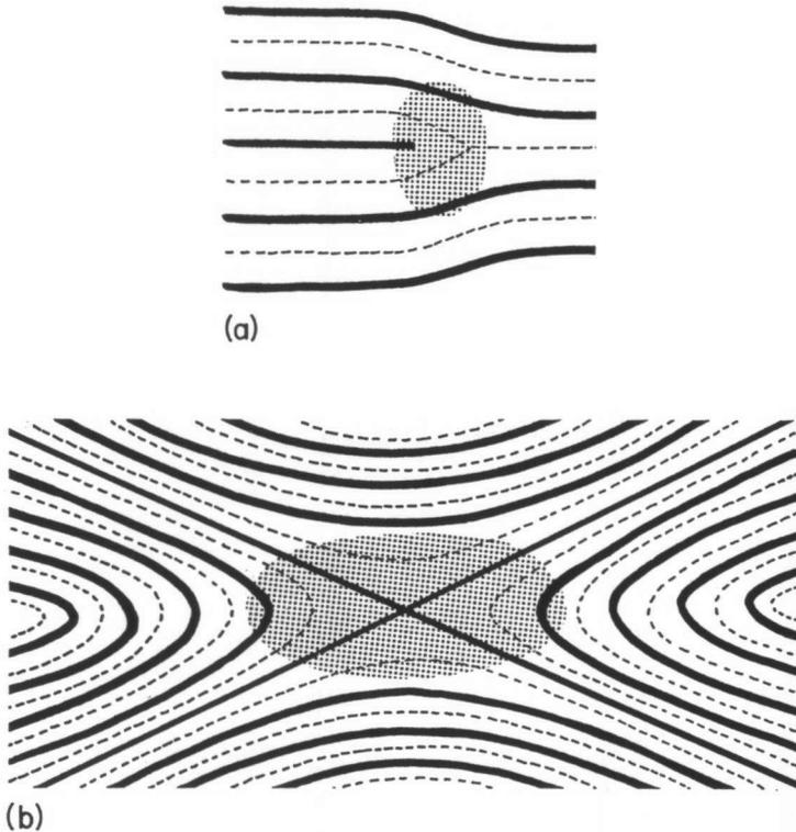
**Fig. 12.** Diagram of two typical defects found in the helicoidal pattern. (a) Edge dislocation. (b) Saddle-like disclination.
