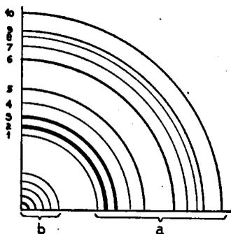
Fig. 1. Diagrammatic representation of a quadrant of the X-ray powder photograph of a normal aliphatic long-chain compound. The intensity of the interference-circles is shown by the width of the lines.
