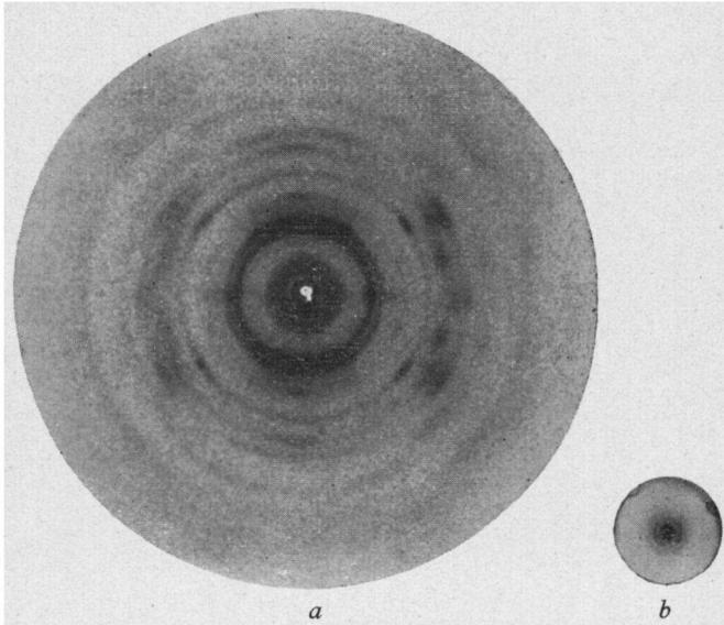
Fig. 20. *a*. Enlarged micro-diagram of a packet of wax rods, obtained with the beam at right angles to the long axis of the rods.
