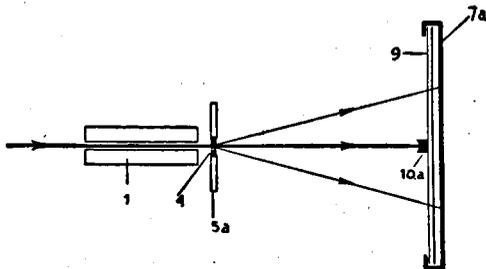
Fig. 5. Principle of X-ray powder photography on flat film.
