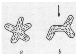
Fig. 26. Cross-sections of rods in which the direction of the crystallite axis with long period is indicated as supposed on account of the observations under the polarising microscope.
