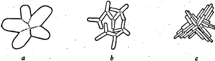
Fig. 27. Possible dimensions and arrangements of crystallites in the wax rods. In the direction perpendicular to the plane of drawing the crystallites are considered to be very elongated. Further explanation is given in the text.
