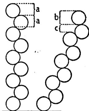
Fig. 3. The increment of the long-chain spacing per carbon atom: a constant amount  $a$  in chains at right angles to the basal plane, or alternating different amounts  $b$  and  $c$  in chains at oblique angles.
