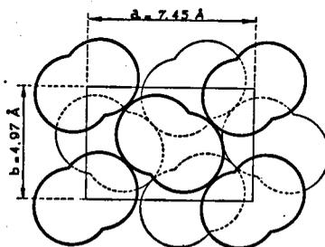
Fig. 2. Diagram showing the crystalline arrangement of the zig-zag chains of carbon atoms in a normal long-chain paraffin (Müller, 1928). Projection viewed along the chain direction. Two layers of chains are shown; those of the upper layer are drawn in heavy lines.
