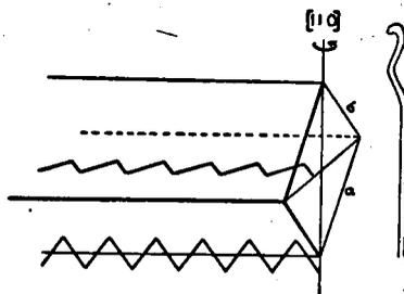
Fig. 23. Orientation of the crystallites in a wax rod according to X-ray evidence.
