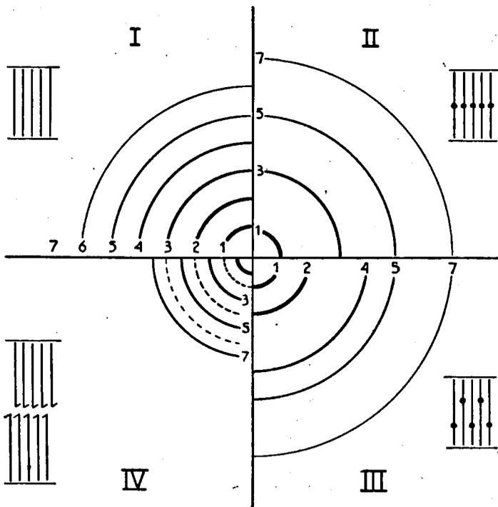
Fig. 4. Diagram showing types of molecules of frequently occurring wax constituents, as placed between the net-planes with long spacing, and their characteristic sets of long-chain reflections. The zig-zag chains are represented by straight lines. The molecules are supposed to possess equal chain lengths and to be crystallised in the rhombic modification.
