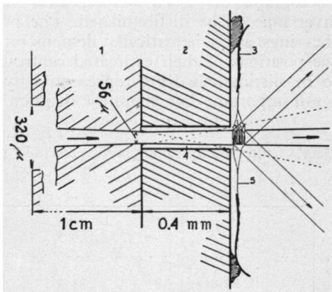
Fig. 21. Method of mounting the specimen when obtaining the photograph shown in fig. 20. Drawing to scale. Explanation is given in the text.
