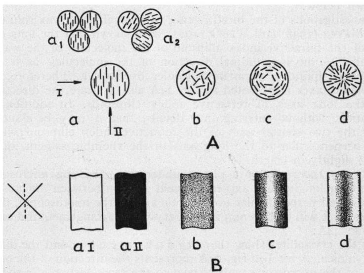
Fig. 24A. Theoretical possibilities of arrangement of the crystallites in the wax rods in directions perpendicular to the longitudinal direction of the rods, represented by indicating the direction of the crystallite axes on the cross-section of the rod. Fig. 24B. The behaviour of a rod placed in diagonal position between crossed nicols for the various arrangements represented in fig. 24A.
