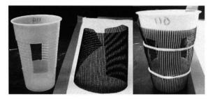
Fig. 1. Housing chamber for libellulid larvae. Chamber is made from a 480 ml (16 oz) plastic drinking cup with  $3 \times 5$  cm windows. The chamber is surrounded by nylon window screen to allow water to flow but retain the larvae. One chamber holds 1-3 larvae.
