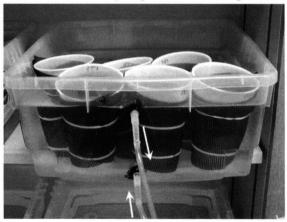
Fig. 2. Translucent box used to contain housing chambers for libellulid larvae. The polyethylene box is  $38 \times 38 \times 16.5$  cm and can hold up to 10 housing chambers (Fig. 1). Arrows indicate flow of water through plastic tubing.
