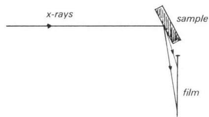
On the flat film the crystal plane reflections are recorded as arcs of circles. In principle three kinds of diagrams can be obtained:
