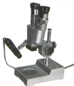
Stereomicroscop STO vergrotingsbereik 5X - 140X
