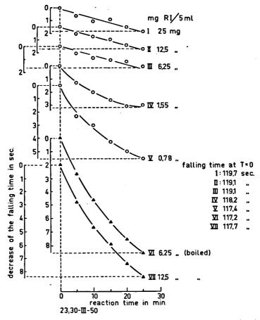
Fig. 8a. The effect of different amounts of inhibitor on the decrease in viscosity of a pectin solution caused by pectinase. 50 ml 0,20 % B.P.-pectin in 0,05 mol. succinic acid-borax buffer, pH 3,6; 5 ml inhibitor solution containing different amounts of RI; 1 ml 1 % Pectasin-A.
