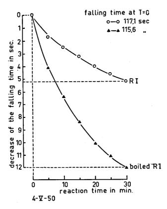
Fig. 11. The effect of the inhibitor on the decrease in viscosity of a pear-pectin solution caused by pectinase.
