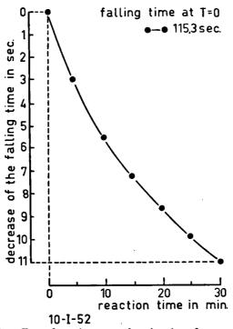
Fig. 1. The effect of pectinase on the viscosity of a pectin solution. 50 ml 0,22 % B.P.-pectin in 0.05 mol. succinic acid-borax buffer, pH 3,6; 1 ml 1 % Pectasin-A. Temp. 25° C.
