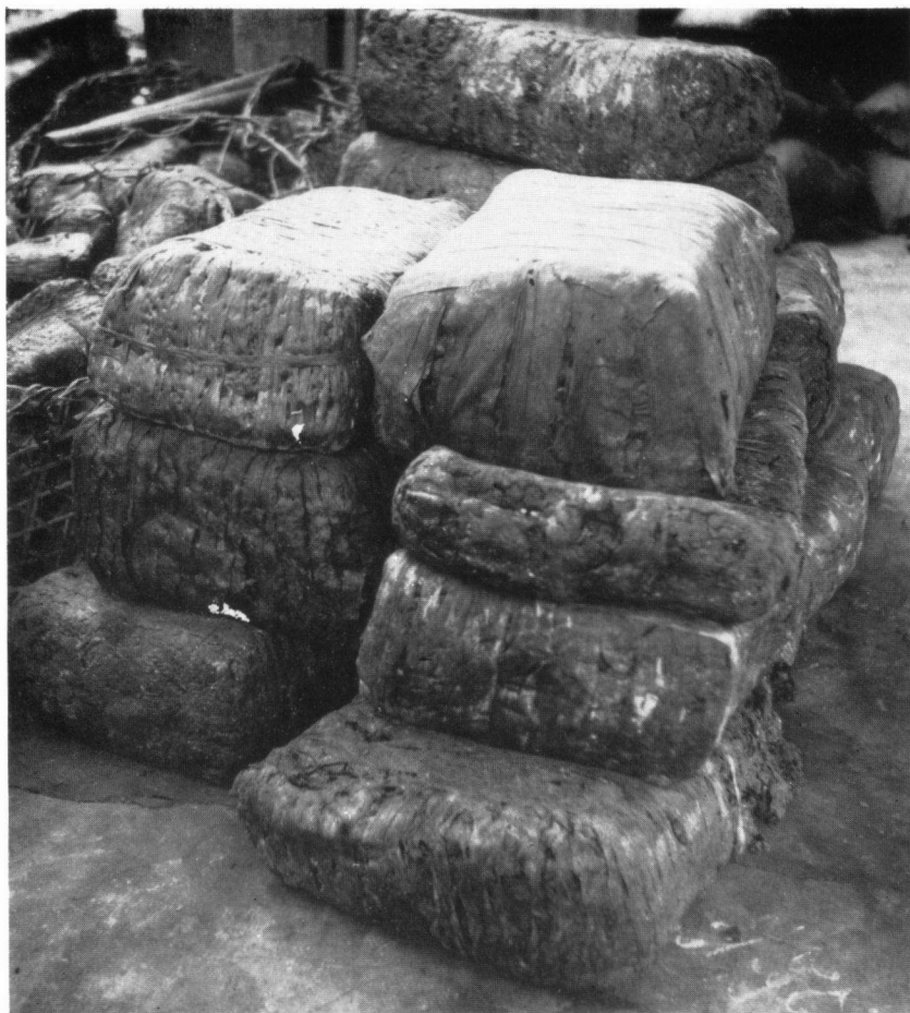
Along the Río Igaraparaná and adjacent rivers, rubber is prepared principally from Hevea guianensis var. lutea in the form of rabos del Putumayo ("Putumayo tails") and Putumayo blocks . In both cases, scrap rubber or sernambí , strips allowed to dry on the tree, are pressed together: in the former, in shapes simulating tails; in the latter, into large blocks, pictured above, made with crude presses. Photographed by R. E. Schultes. Río Igaraparaná, Colombia.
