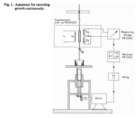
recorder pen switches on a motor. The table on which the plant is fixed moves down over 1mm, the motor is switched off when the recorder pen reaches the beginning of the scale. In this way growth can be recorded for a longer period.
