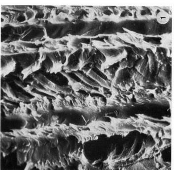
Fig. 2. 'Soft-rot' destruction in the secondary wall, showing the characteristic pointed ends of the cavity, in which a hypha fragment is still pre-Fibre tracheids of a wood sample of Dicranostyles mildbraediana attacked by 'soft-rot' fungus. Fig. 1. Cavities in the walls follow the direction of the cellulose microfibrils  $\times$  2000.
