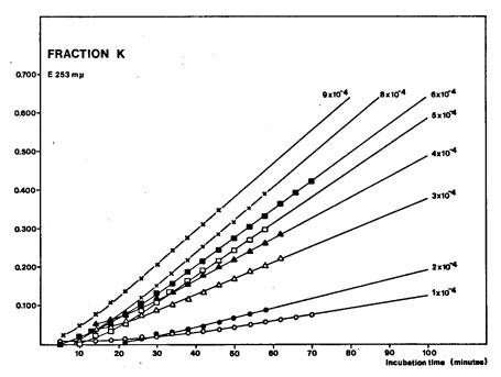
Fig. 4. Time curves of IAA-oxidase activity expressed as increase in optical density at 253 m $\mu$ . The enzyme dilutions tested are given for each curve.
