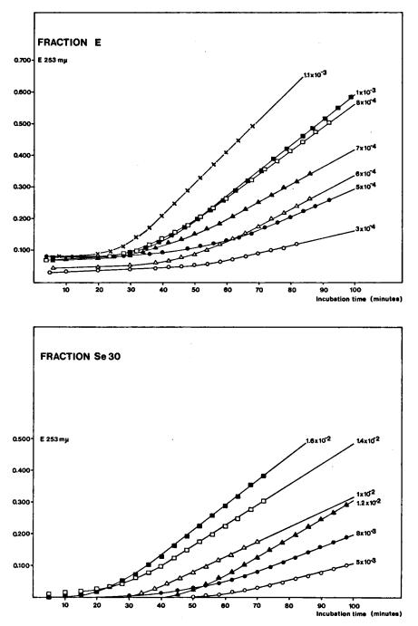
Fig. 1. Time curves of IAA-oxidase activity expressed as increase in optical density at 253 m $\mu$ .
