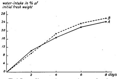
Fig. 9. The influence of hetero-auxin, concentration 1 to 10<sup>7</sup>, on the waterintake. (exp. 235 of table 15). A: distilled water. B: hetero-auxin solution.
