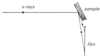
On the flat film the crystal plane reflections are recorded as arcs of circles. In principle three kinds of diagrams can be obtained:
