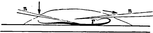
Fig. 3. Diagrammatic representation of the handling of a radula (r) in a drop of liquid on a microscope slide. The radula is pressed down and held in place by one needle (n, left) while the other needle (n, right) is used to smooth out the radula. Both needles are kept in an almost horizontal position.
