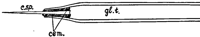
Fig. 2. A cactus spine (c. sp.) mounted in a piece of glass tubing (gl. t.) by means of a cementing substance (cem.). About natural size.
